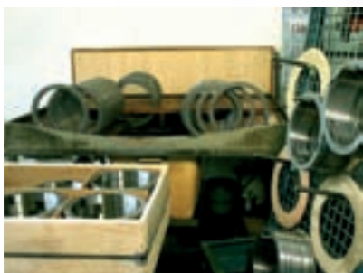
15. Rotary slitter knives and spacers
