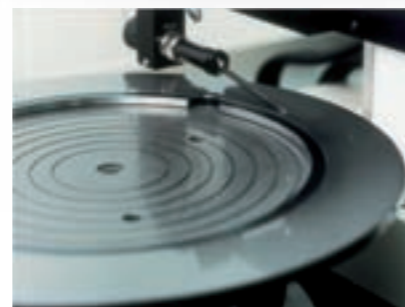
12. Final inspection of flatness of rotary slitter knives
