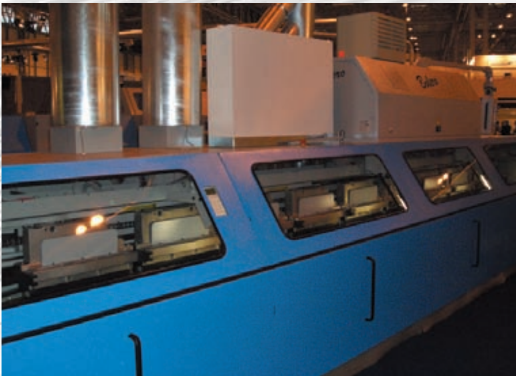
Perfect Binder / Adhesive Binding Machine
